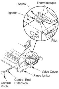
Figure 11 - Installing Cover, Control Knob, and Piezo Ignitor
